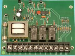
The Digital Sequence Controller is designed for flexibility, adjustability, maintenance, and troubleshooting. The unit can operate in standard cycles or in a shortened test mode, the timing sequences can be manually advanced by a qualified technician for troubleshooting. The controller has dual modes that can be switched between heat type and heatless control cycles.
