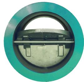
Over time all valve seals experience wear. If a valve design uses the sealing medium as a hinge or sealing surface, wear could cause a catastrophic failure, which can cause the compressed air system to depressurize. The Sullivan-Palatek wafer style check valve utilizes the soft seat only to ensure a bubble tight seal, the primary sealing surface is metal to metal, thus removing the probability of a catastrophic failure.
