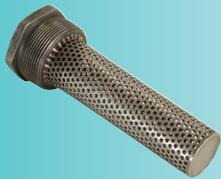
The Sullivan-Palatek desiccant support screens are fabricated from heavy gauge perforated stainless steel. The perforation pattern is designed to retain the desiccant bed while allowing small particles to pass, this prevents particle buildup and high pressure drops. Screens with tighter perforations or wire mesh covers run a high probability of damage from pressure drop. The screens are 100% welded construction, with no epoxy or gluing.
