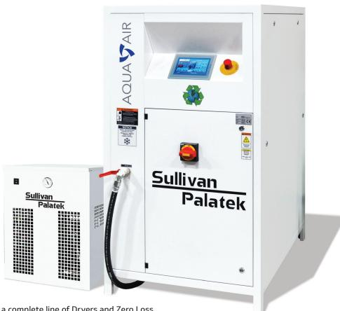
Sullivan-Palatek has a complete line of Dryers and Zero Loss Drains that will be quoted with each compressor package.
